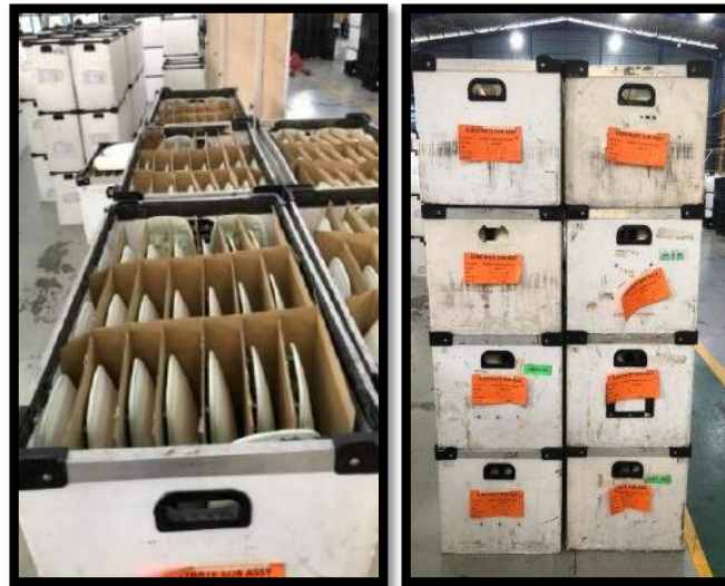
Figure 6: Lucid Substrate Sub Assembly Armrest stacked for Mullen test
