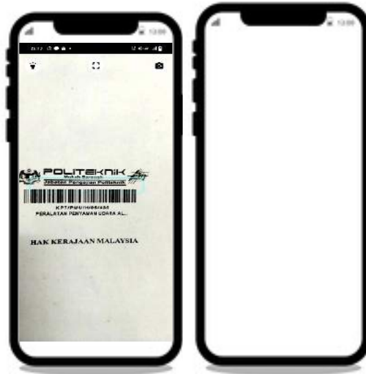
Figure 4: The application tracks the asset details through handphone scanner by scanning the barcode
